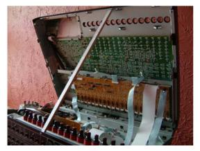
The top of the DA7 is hinged to the base. The hinges are at the front. Remove all small screws along sides, rear top and front top. Then pull MONITOR A LEVEL, MONITOR B LEVEL and TB LEVEL knobs. The top can now be easily lifted from the rear. Use that 50cm long piece of wood to hold the top open as shown opposite.
